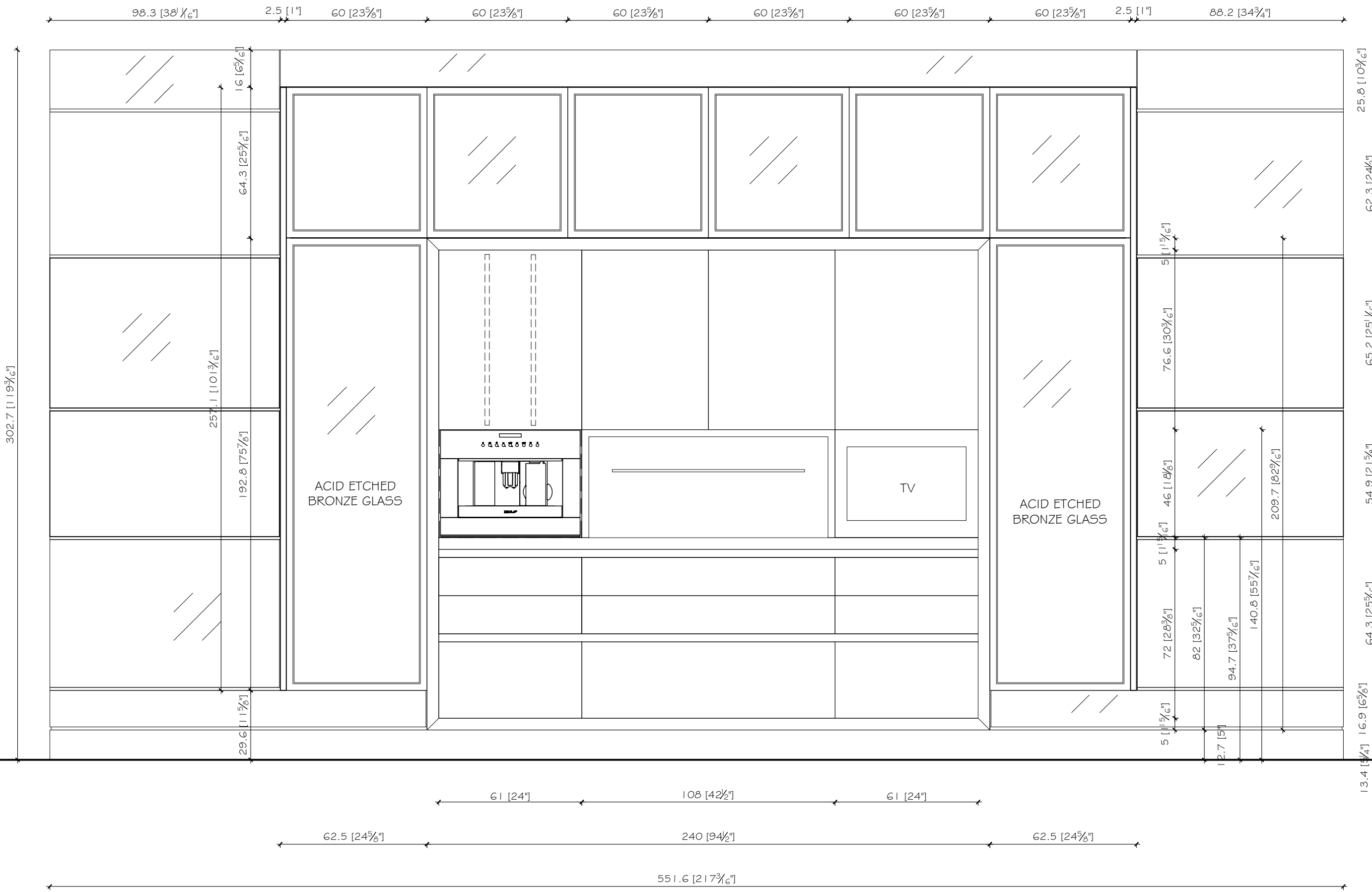
1 A2 EAST ELEVATIONS: WALL PANELS APPLIANCE WALL
